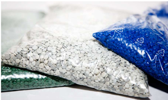
Soft polyethylene granules - source material for new plastic film
